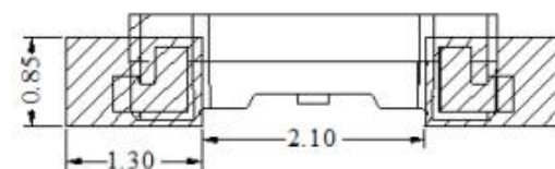
Recommended soldering pad design
